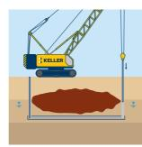
Containment – enclosure around the contaminated zone
